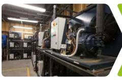
Williams Refrigeration's pass through blast chillers and freezers produce waste heat as a result of the chilling process
